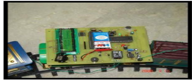
Fig.8. PCB mounted on the engine of the train.
