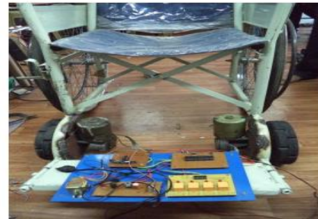
Fig 10. Voice Controlled Wheelchair
