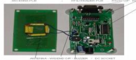
Figure 3 Inside RFID Reader
