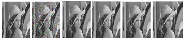
Fig: 1 Results of different algorithms for Lena image.(A) input image,(B)noisy image,(c)SMF image,(D) AMF image,(E) MDBUTMF image,(F) Weighted Median Filter image.
