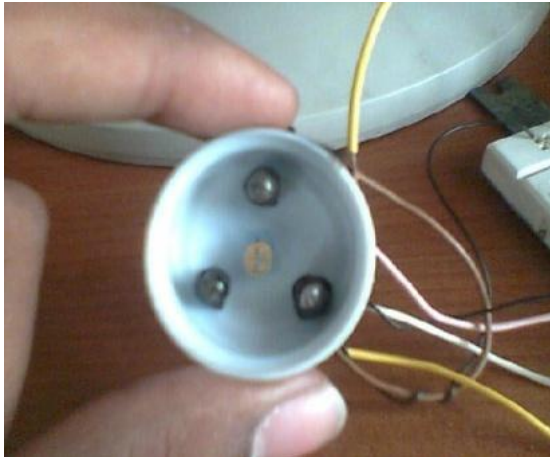
Fig. 8 Sensor unit design to measure pH level
