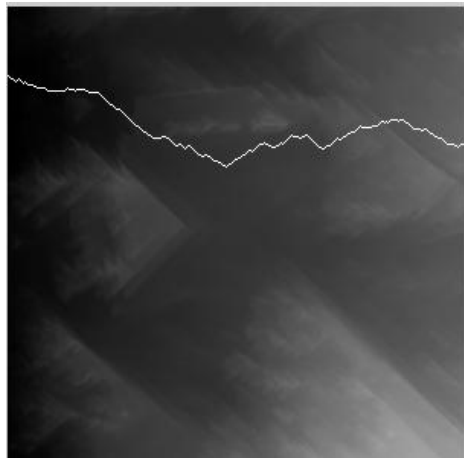
Fig 4: energy map with horizontal seam
