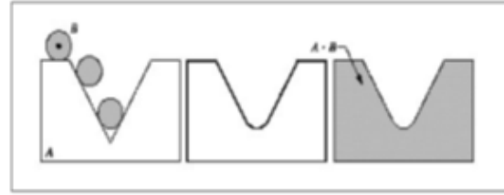
Figure 2.9: Illustration of Binary Closing Process [13]
